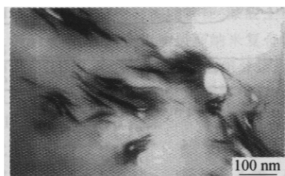
Fig. 3 Transmission electron micrographs of the sPS/PA6/S s PS-H/MTN-S s PS (62/20/5/6 ~ 18 wt) nanocomposite
